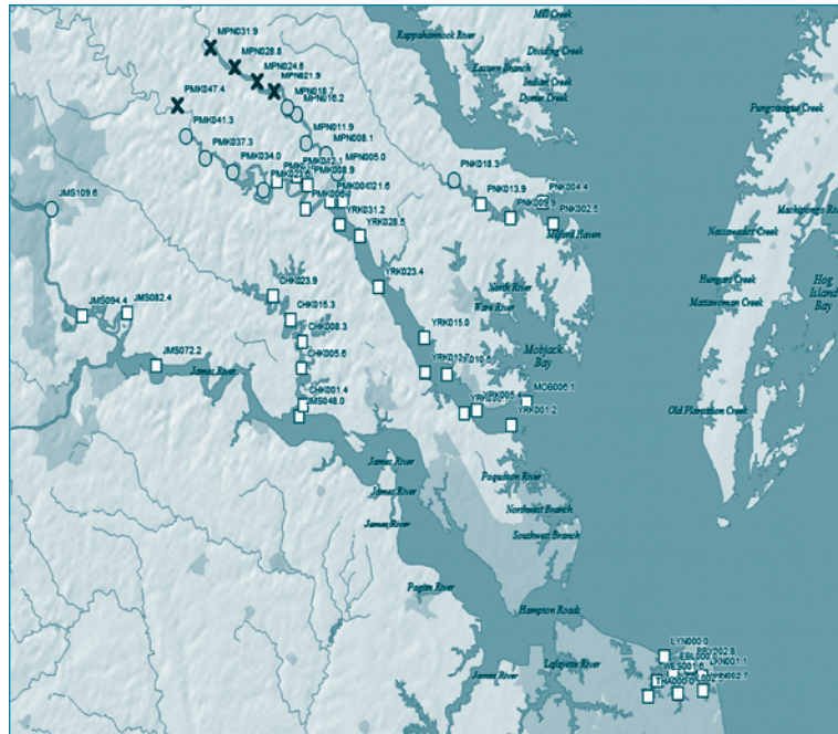
Figure VII-12. Locations of the Virginia Chesapeake Bay Shallow-water Monitoring Program calibration stations. In each location, a circle indicates that no significant difference occurs between the in situ chlorophyll measures and the in vitro chlorophyll measures. A square indicates that the in situ measures are less than the in vitro measures. An X indicates that in-situ measures are greater than the in-vitro measures.
